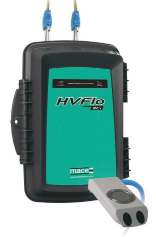
HVFlo XCi is a high performance battery operated open channel flow monitoring solution for wastewater, stormwater and industrial discharge applications
