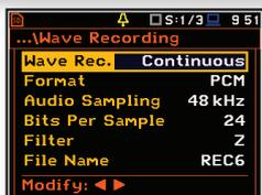
Time signal recording means recording the raw signal samples with defined frequency up to 48 kHz. Analysis of the raw signal is used whenever frequency analysis is not sufficient. Post-processing of wave files such as calculation of tonality is available in SvanPC++ program. Time signal is recorded in a wave format which means that it can be played back in the PC software and used for noise source recognition (audio recording).
